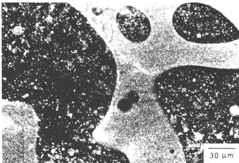
Figures 3a, 3b, 3c. (a) (above) Optical micrograph of the microtomed section of a 50/50 PC-PST blend. (b) (top right) Scanning electron micrograph of the PST phase in the 50/50 PC-PST blend. (c) (bottom right) Scanning electron micrograph of the etched fracture surface of the 50/50 PC-PST blend showing both continuous phases.
